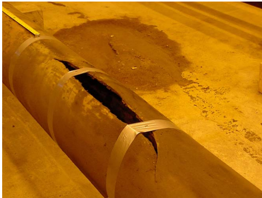
Figure 4: Damaged surface casing recovered from Well A-22
