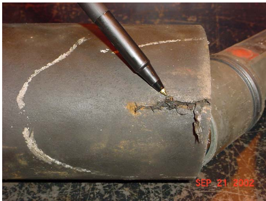
Figure 3: Well A-22 tubing split
